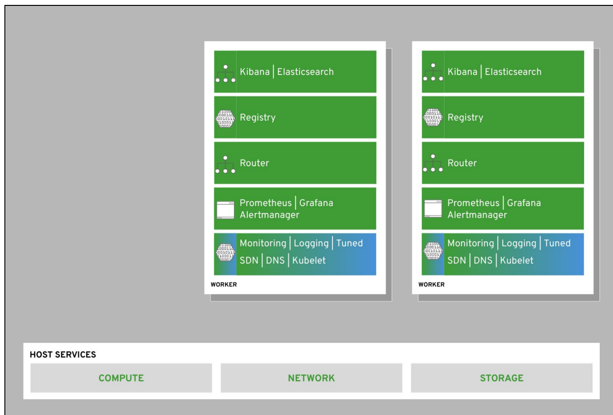
Figure 3-2: The OpenShift Worker Components (Worker Services May Vary for Each Worker Instance; Other Workers Services Are Not Shown Here)
